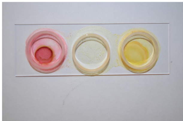
Fig. 1. A) Left-most spot test with double-base powder. B) Middle spot test with reagent control. C) Right most spot test with single-base powder.
