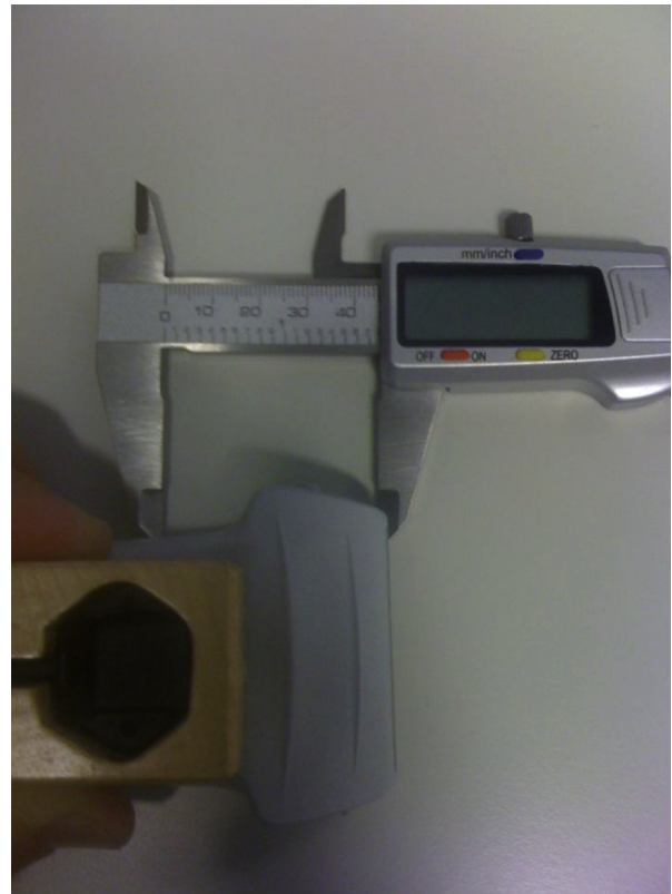
Fig. 1. The electromagnetic sensor (black hexagonal) was fixed, using a specific wooden piece, to the top of the transducer to avoid interference, and the source transmitter was mounted in front of the patients.
