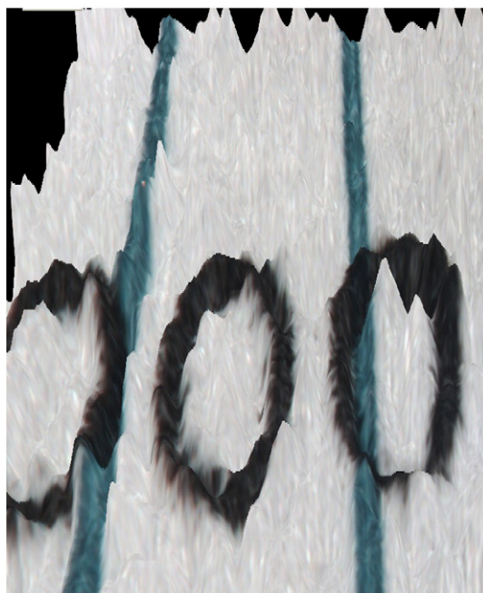
Fig. 2. Showing transformed 2D image of black typewriter stroke intersected by green gel pen stroke into 3D image.
