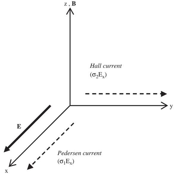
Fig. 1. Pedersen and Hall currents resulting from an electric field  $\mathbf{E}$  in the  $+x$ -direction. The magnetic field is directed along the  $+z$ -axis.
