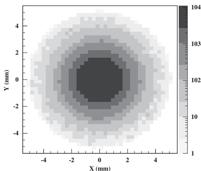
Fig. 1. Two-dimensional beam distribution, 6 cm away from the extraction window.
