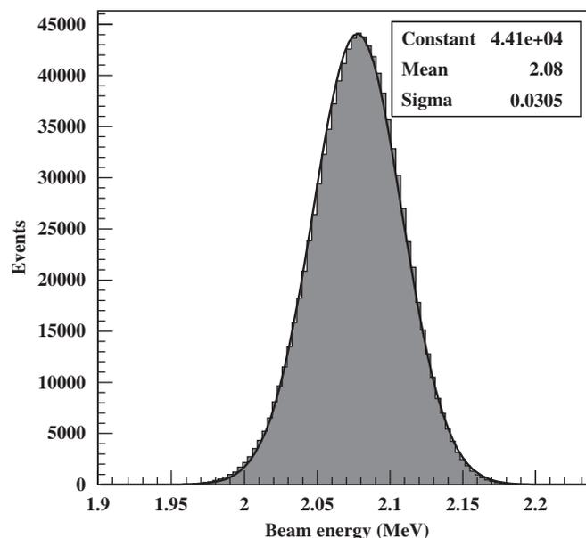
Fig. 2. Beam energy distribution at sample position. A Gaussian fit to the distribution is shown giving a mean value of 2.06 MeV. The fit parameters are given in the top right inset.
