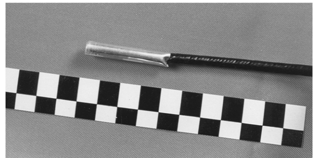
Fig. 6. Detonation cap photographed with measure tape.
