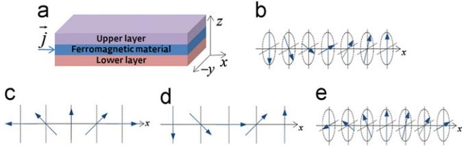
**Fig. 1.** (a) A film geometry and a coordinate convention. A magnetic configuration of (b) Bloch ( $\hat{z}$ ) wall, (c) Néel ( $\hat{x}$ ) wall, (d) Néel ( $\hat{z}$ ) wall, and (e) Bloch ( $\hat{y}$ ) wall.
