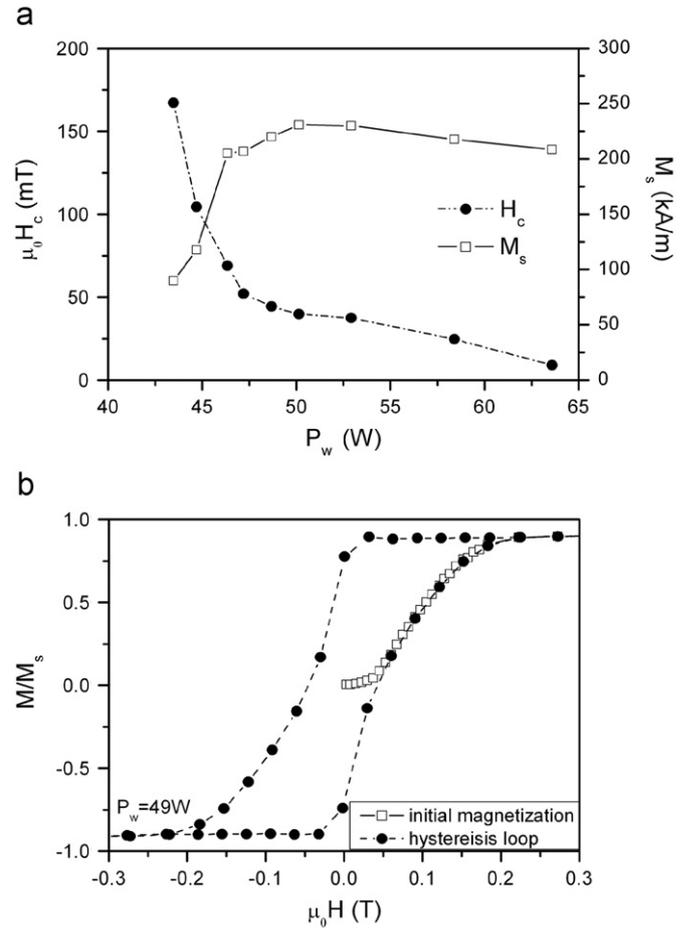
Fig. 2. (a) Variation of out-of-plane coercivity  $\mu_0 H_c$  and saturation magnetization  $M_s$  with dc power  $P_w$ . (b) Initial magnetization curve and magnetic hysteresis loop.
