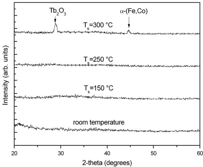
Fig. 1. XRD patterns of the Tb<sub>40</sub>(FeCoV)<sub>60</sub> films deposited at varied substrate temperatures.
