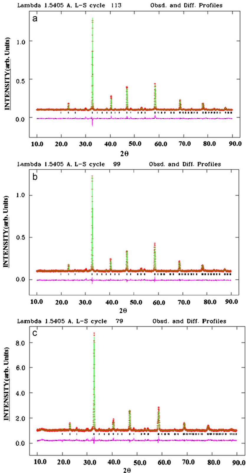
Fig. 1. Refined XRD pattern for (a) LCMVDy<sub>0.03</sub>, (b) LCMVDy<sub>0.15</sub> and (c) LCMVDy<sub>0.25</sub>. The plot at the bottom is the difference between the calculated and observed intensities.
