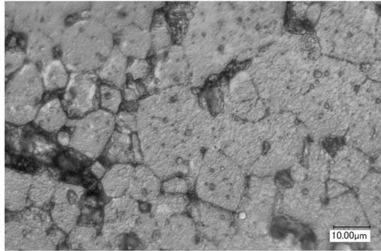
Fig. 1. The microstructure of the sintered Nd-Fe-B magnet.
