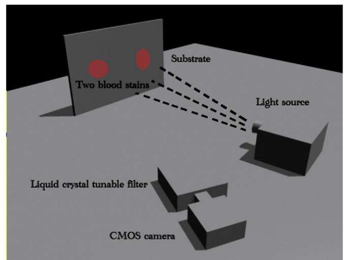
Fig. 1. A schematic of the hyperspectral imaging system.
