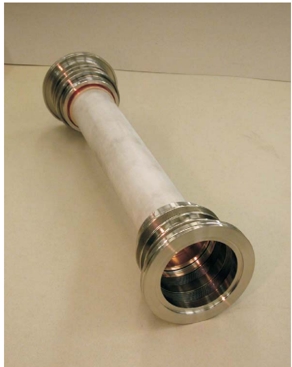
Fig. 1. Ceramic vacuum chamber with integrated bellows for the fast kicker magnet.
