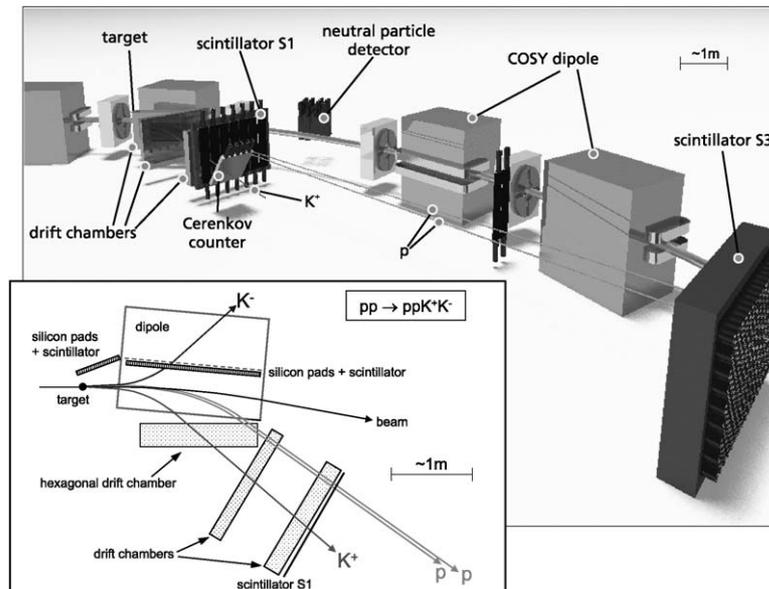
Fig. 1. The experiment COSY-11 with the main components. The overlaid box shows a schematic view for an exemplary event of the reaction channel  $pp \rightarrow ppK^+K^-$ . The sudden stop of the kaon track in the three-dimensional picture indicates its decay.
