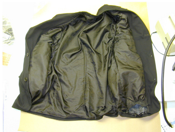
Fig. 3. Gross heat damage to the lining along the hem of a jacket.
