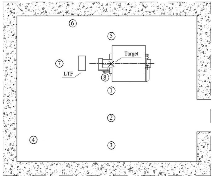
**Figure 2.** Sampling positions adopted during the measurement campaign within the bunker.
