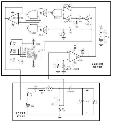
Fig. 1. Experimental current-programmed boost converter.
