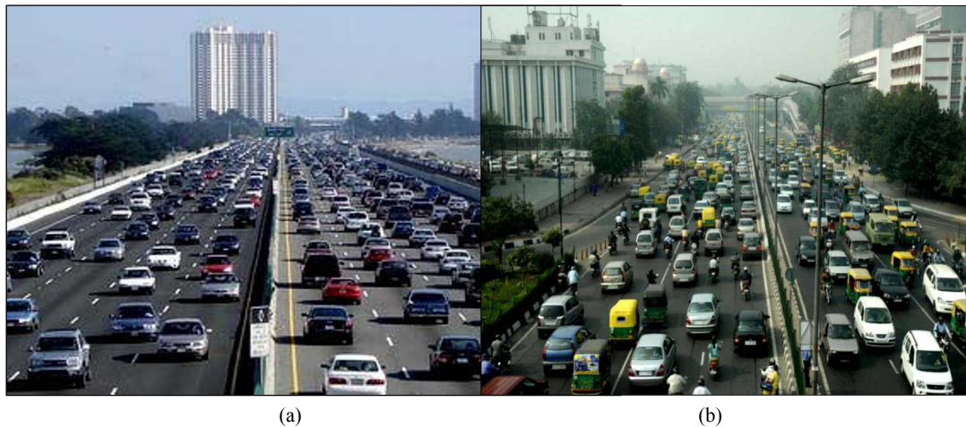
Fig. 1 Traffic flow under different types of traffic condition (a: homogeneous traffic; b: heterogeneous traffic)
