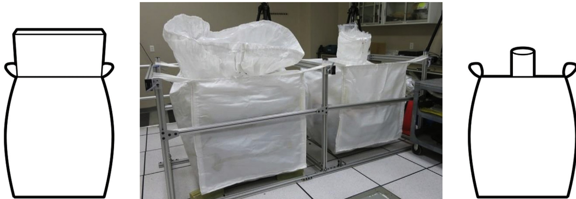
Fig. 1. Type of bags used; drawing of duffel (left), lab setup of duffel and spout, and drawing of spout (right).
