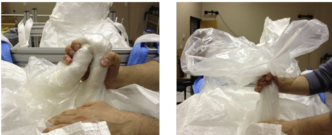
Fig. 2. Bag closing methods; snaking (left), flowering (right).
