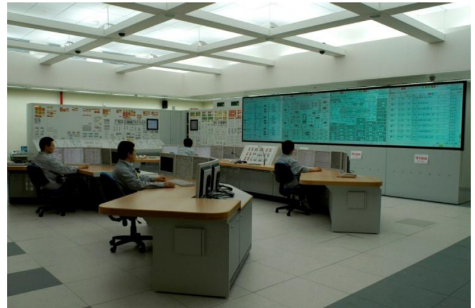
Fig. 2. Ling-Ao Phase II full scope simulator (Source: Ling-Ao NPP).
