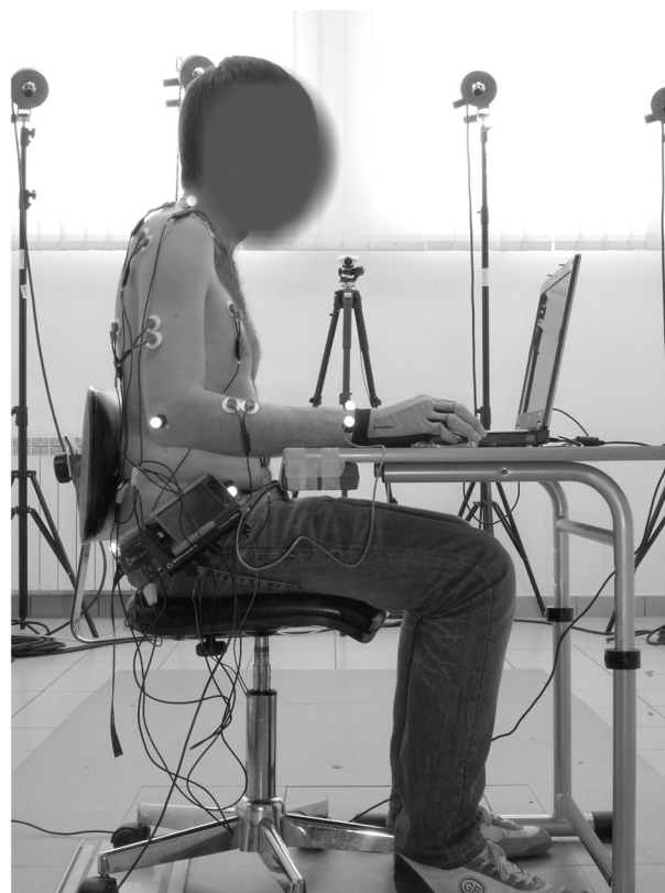
Fig. 1. A representative picture of the position of the reflective markers and electrodes with video recording equipment.
