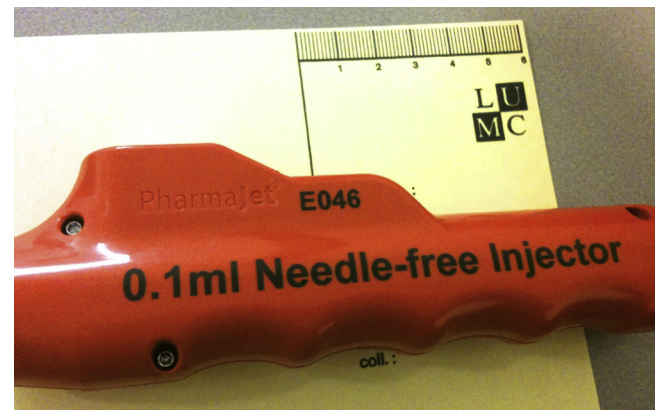
Photograph 1. PharmaJet Needle-free Jet Injection System for intradermal delivery. The ID injector used in this study was an investigational version of the FDA 510k-cleared v1.0 SC/IM device.
