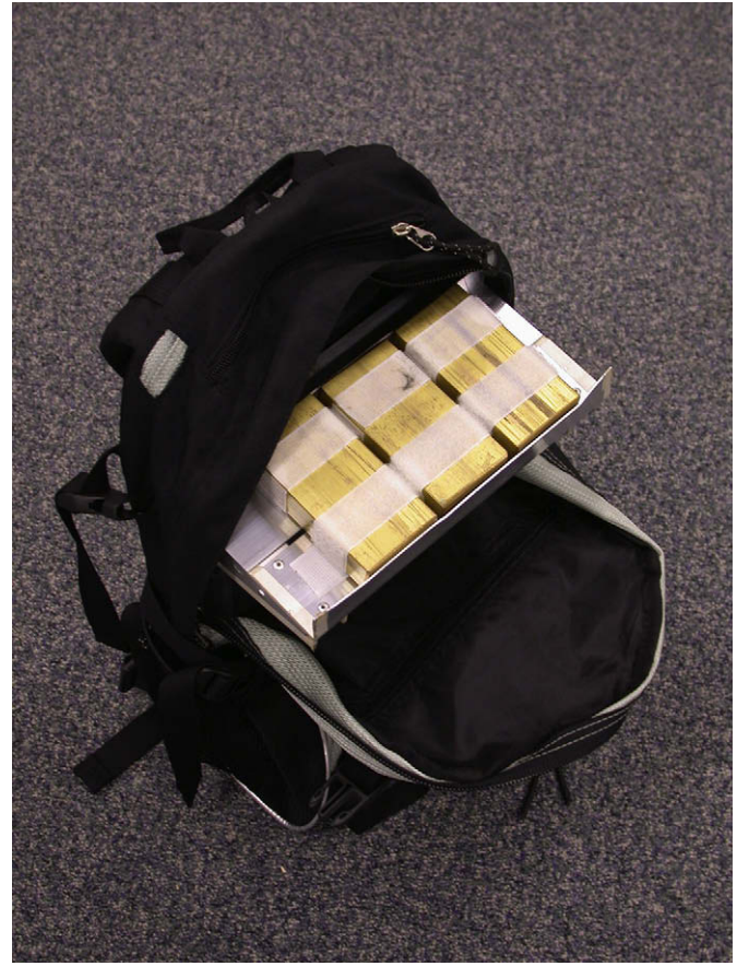
Fig. 1. Testing backpack with an internal frame for adjusting the position of the center of gravity of the load.
