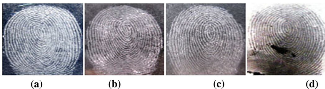
Figure 2 Showing comparative visualization of latent fingerprints on glass surface with silica gel G powder (a) white powder (b) light grey powder (c) black powder (d).
