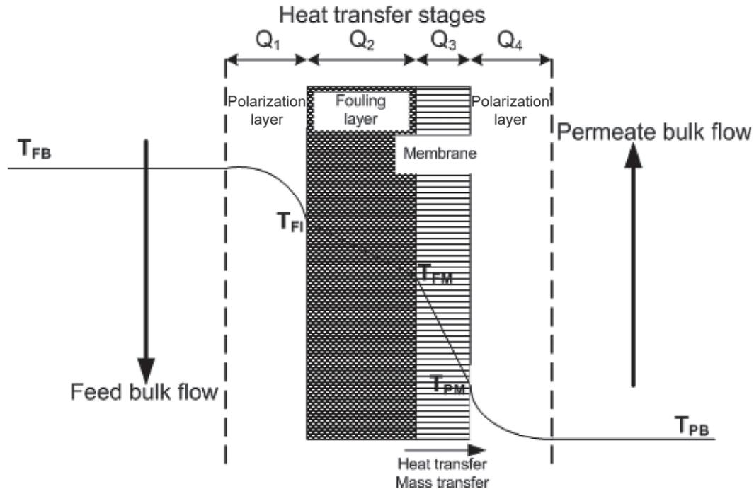
**Figure 1.** Temperature profile across the membrane in a typical direct-contact membrane distillation (DMCD) process.  $Q$  = heat transfer;  $T_{FB}$  = temperature of feed bulk;  $T_{Fl}$  = temperature of fouling layer;  $T_{FM}$  = temperature of feed membrane;  $T_{PM}$  = temperature of permeate membrane;  $T_{PB}$  = temperature of permeate bulk.
