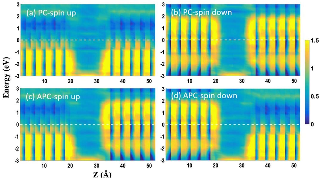
Fig. 2. Project density of states (PDOS) by different colors on a logarithmic scale along the transport direction ( $z$ -axis) of the  $\text{Fe}_4\text{N}/\text{Ag}/\text{Fe}_4\text{N}$  CPP-SV at equilibrium.
