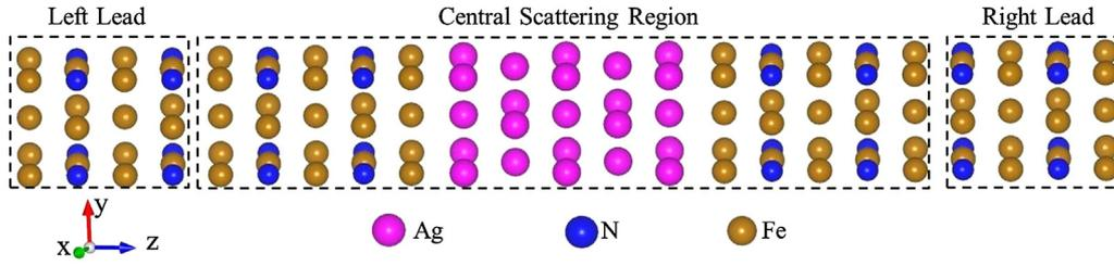
Fig. 1. Schematic illustration of the  $\text{Fe}_4\text{N}/\text{Ag}/\text{Fe}_4\text{N}$  CPP-SV. The  $z$ -axis is the transport direction.
