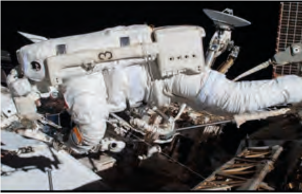
Figure 1. Extravehicular Mobility Unit (EMU)
