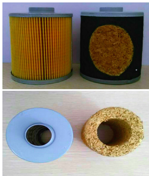
Fig. 1. Appearance of conventional fiber-paper filter (left) and modified sawdust oil filter (right).
