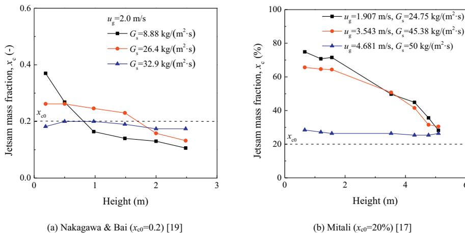
Fig. 1. Jetsam mass fraction along the riser height in the literature.
