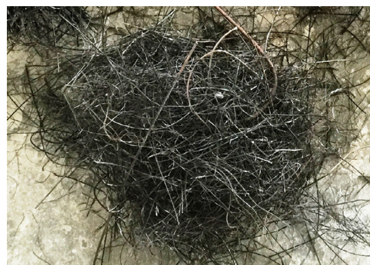
Fig. 1. Waste steel fibers used in the study.
