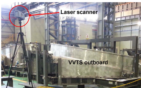
Fig. 3. 3D scanning of VVTS outboard upper segment.
