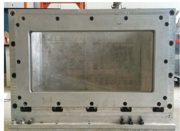
Fig. 3. Rigid container used in the test: (a) structure diagram; (b) photo.
