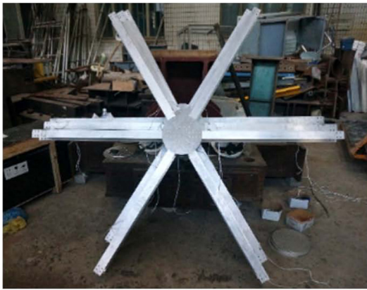
Fig. 1. AAG joint specimens. (a) Configuration. (b) Specimens with shear connectors.
