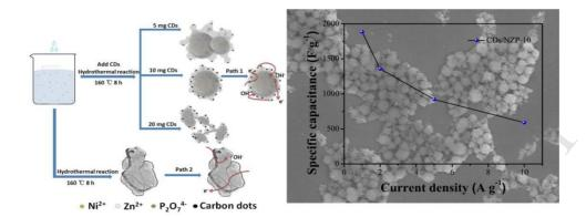
Mulberry-like nickel-zinc phosphate composite decorated with carbon dots was synthesized and employed for high-performance supercapacitor electrode.
