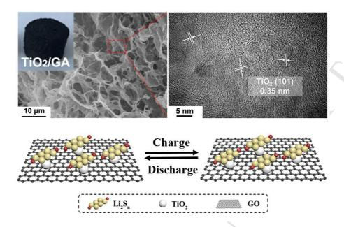
A three-dimensional  $TiO_2$ /graphene aerogel ( $TiO_2$ /GA) composite with hierarchical porous structure, showing strong interfacial chemical and physical interactions with soluble polysulfide intermediates ( $Li_2S_n$ ,  $4 \le n \le 8$ ), is effectively applied as a promising anchoring material for lithium–sulfur batteries.
