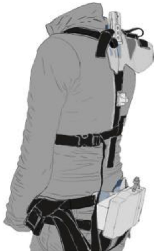
Fig. 1. Posture dosimeter. This equipment is composed of three parts: two inertial sensors (Xsens Technologies B.V., NL) on the pelvis (lower sensor) and on the thorax (upper sensor) and a flexible structure equipped with a potentiometer that connects the two orientation sensors (Plamondon et al., 2007). Data from the two sensors and the potentiometer are integrated with a complementary filter that optimizes the sensors' response (Plamondon et al., 2007).
