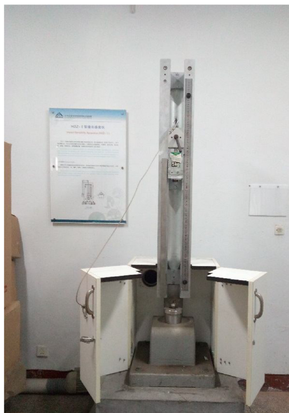
Fig. 2. The drop weight test device.
