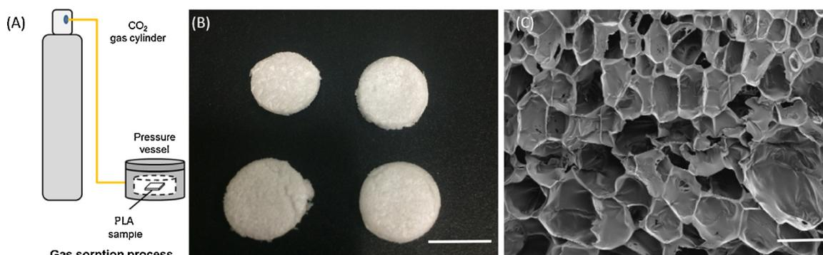
Fig. 1. PLA scaffolds fabrication. (A) PLA scaffold fabricated by solvent-free solid-state-foaming approach. (B) Disk-shaped PLA scaffolds. Scale bar: 10 mm. (C) Cross section of scanning electron microscopic (SEM) image of a PLA scaffold. Scale bar: 500 μm.
