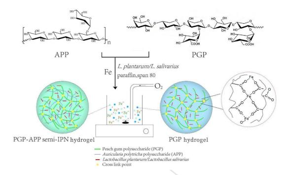
A Schematic illustration of the fabrication of the PGP hydrogel and PGP-APP semi-IPN hydrogel.
