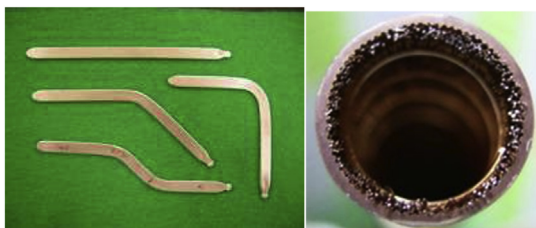
Fig. 2. Flattened copper-water heat pipes (left) and a heat pipe cross section showing wick structure along the inner periphery (right).
