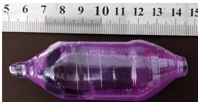
Fig. 3. The photograph of as-grown Nd:Gd 0.69 Y 0.3 TaO 4 mixed crystal.
