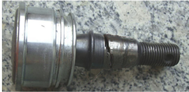
Fig. 1. Fractured balance ball pin.
