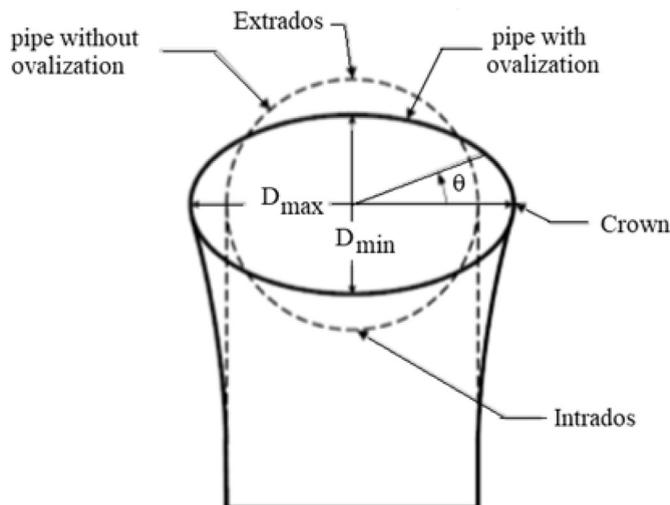
Fig. 2. Definition of minimum and maximum diameter for the flattening parameter.
