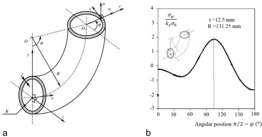
Fig. 1. a: Geometrical dimensions of a curved pipe. b non-dimensional hoop stress  $\frac{\sigma_\phi}{k_z\sigma_0}$  versus angular position
