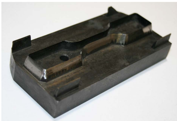
Fig. 2. Blanking die used in the process of cutting out specimens from heat-shrinkable film.
