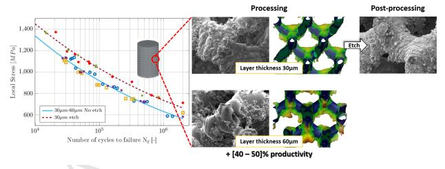
Keywords: laser powder bed fusion, CoCr, fatigue, layer thickness, (increased) productivity
