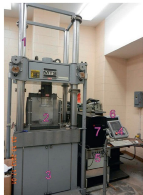
Fig. 2. MTS servo-controlled compression testing machine and its components: (1) Machine load, (2) Glass shield, (3) Hydraulic actuator, (4) Manual control system, (5) Strain gauge control panel, (6) Computer, (7) MTS data acquisition system. 15
