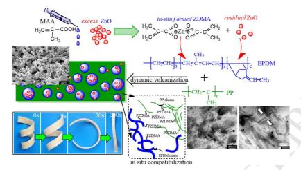
Design of shape-memory materials based on sea-island structured EPDM/PP
