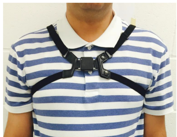
Fig. 1. Inertial sensor strapped on the chest to assess trunk posture.
