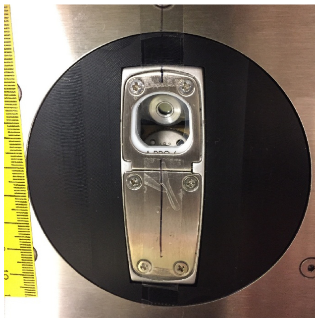
Fig. 2. The open beam configuration showing the location where samples are placed.
