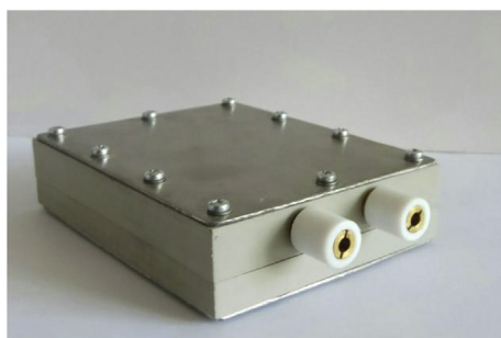
Fig. 2. Photo of a prismatic dismountable cell case.
