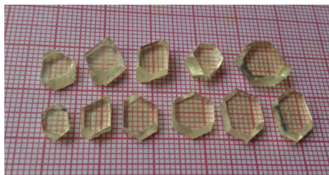
Fig. 2. As grown AMP4N single crystal.
